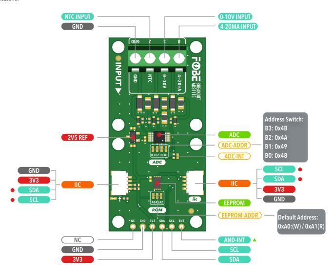
4-channel 16-bit ADC converter
