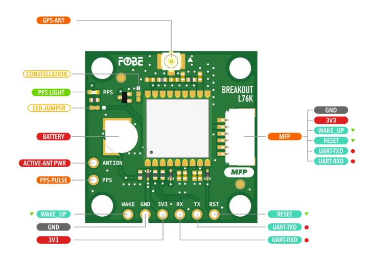
${\tt BATTERY: Build-in\ 3.1V\ Rechargeable\ Button\ Cell\ Battery\ for\ Data\ Retention}$
