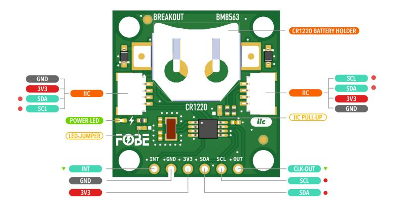
INT: Trigger when the programmed timing conditions are met
